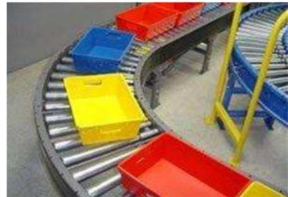
Materials handling includes all movement of materials, in a manufacturing situation. It has been defined by the Materials Handling Division, American Society of Mechanical Engineers, as follows: “Materials handling is the art and science involving the moving, packing, and storing of substances in any form.”
